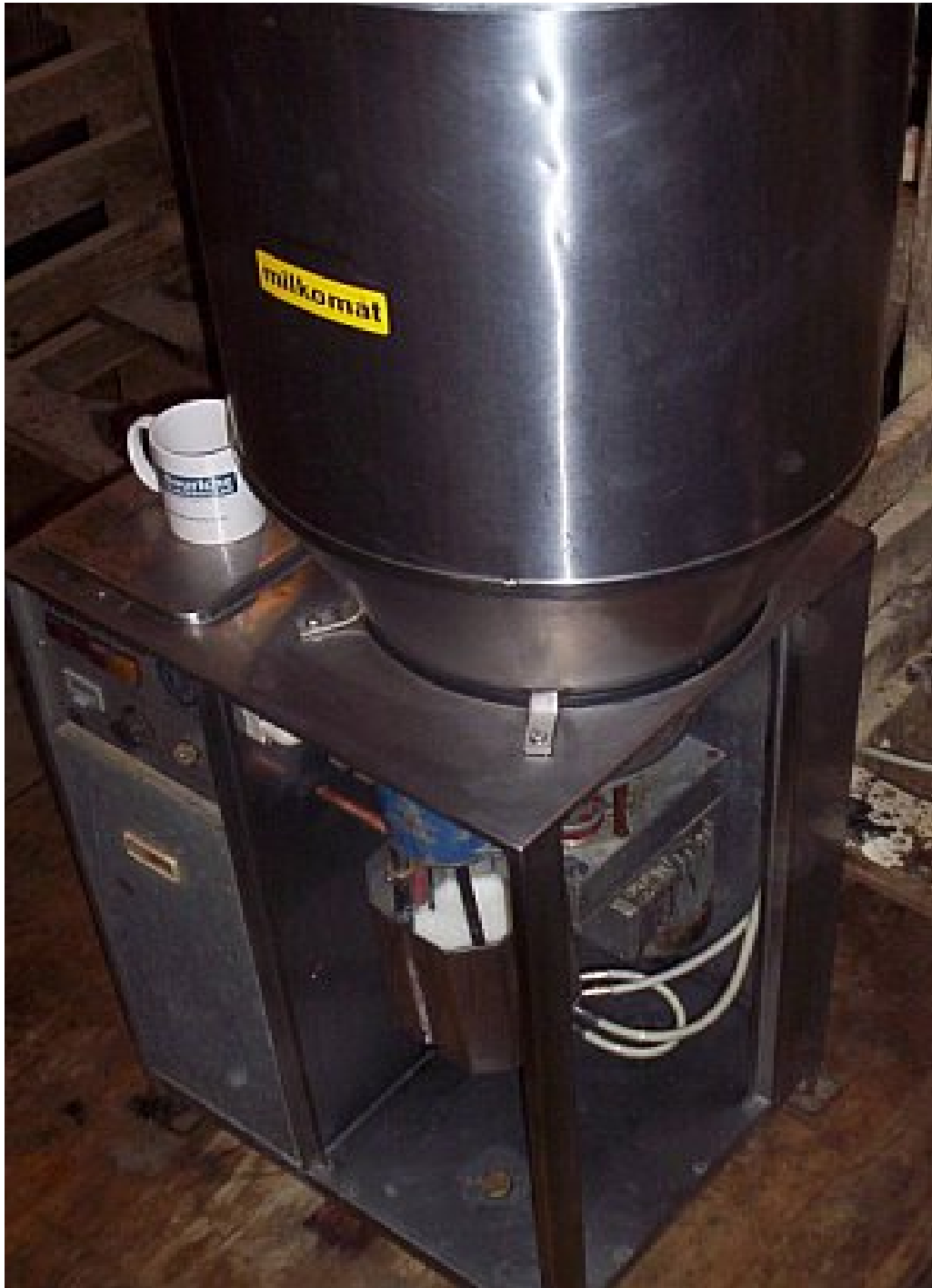
Figure 3. Milkomat free-choice system used for veal calves for nearly 25 years in U.S.
