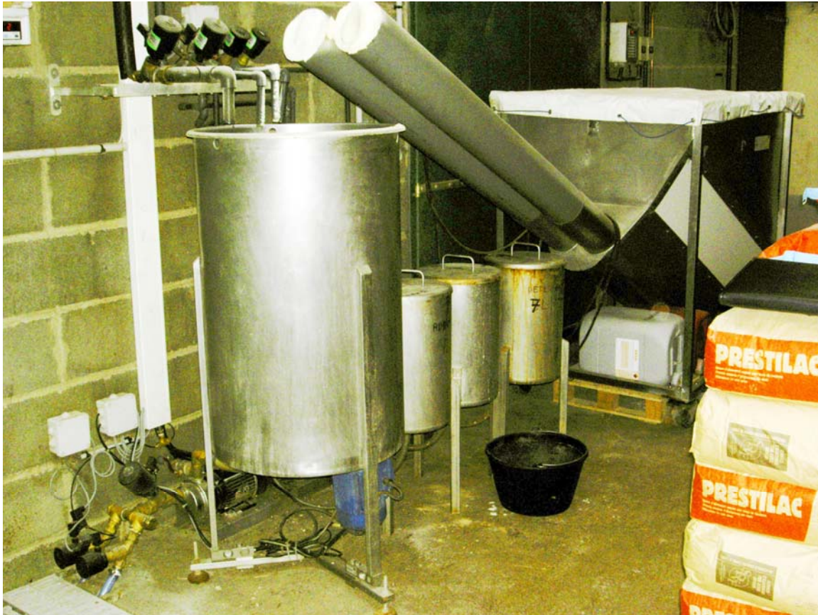
Fig. 2. Cornelli Turbo-Lait system (R to L): double hopper, additive tanks, mixer
