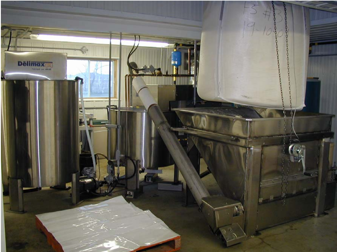
Fig. 1. Delimax Automat system (R to L): tote sac of milk replacer, hopper, mixer, storage tank
