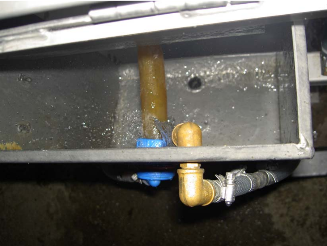
Figure 8. Nipple Being Washed in Feeding Station with Automatic Nipple Washing
